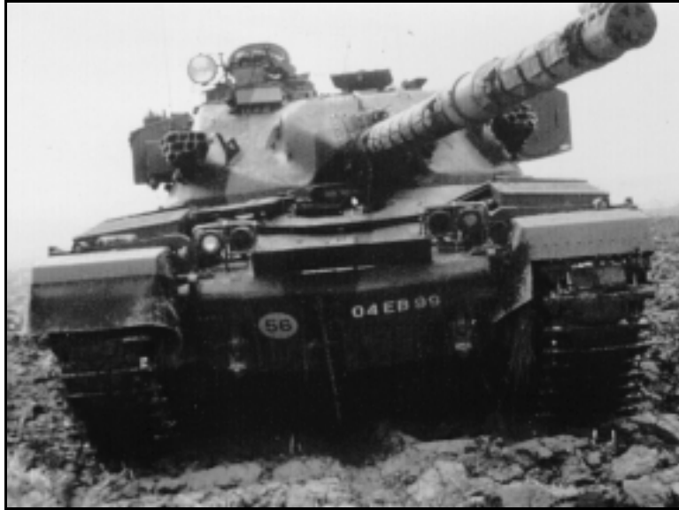
The Kuwaitis fought the Battle of the Bridges with the British Chieftain MBT, at left, equipped with an excellent 120-mm rifled gun, but cursed by power train reliability problems. Infantry carriers include the Soviet BMP, above, and the U.S.-built M113.
